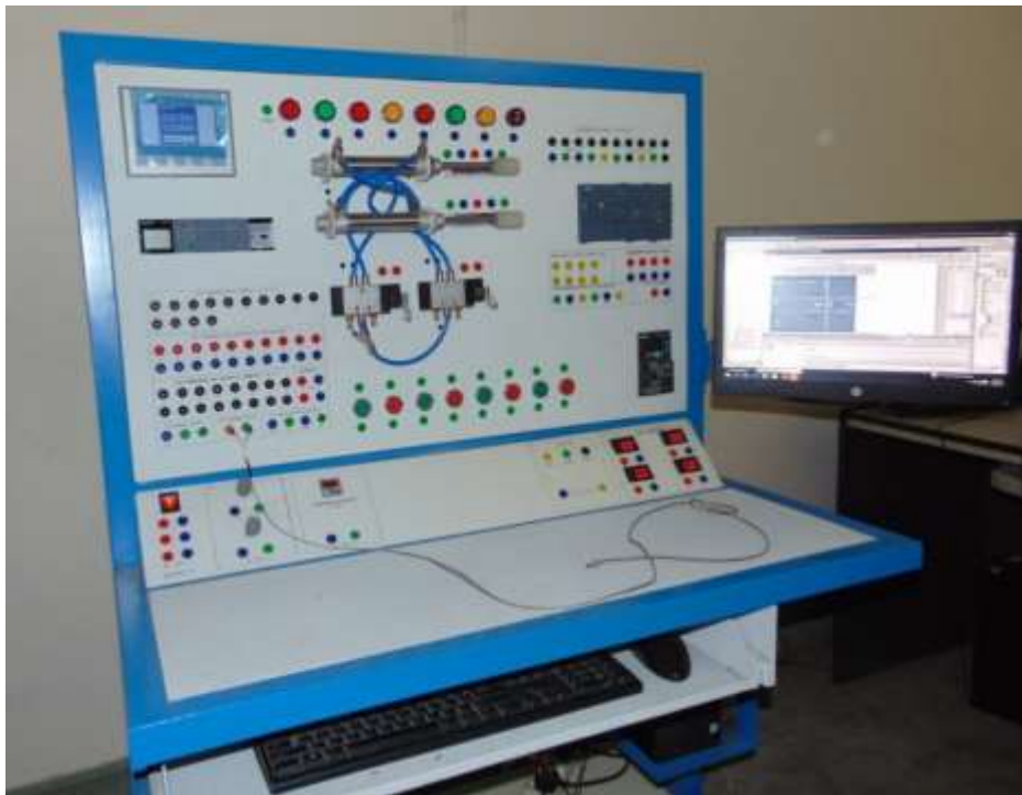
Fig. 07: PLC Advanced work station
